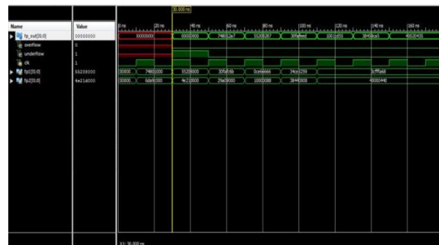
Fig.10: Floating point adder with 2 stage pipelining unit
